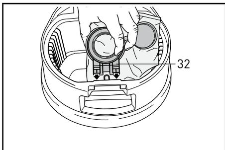
Vacuuming fine dust may require an earlier filter bag change even though the filter bag is not full. Fluff may overfill the filter bag without the light coming on. The bag full indicator only works correctly at full power. At lower levels, the indicator might not indicate correctly. Therefore please check the status regularly at full power.
